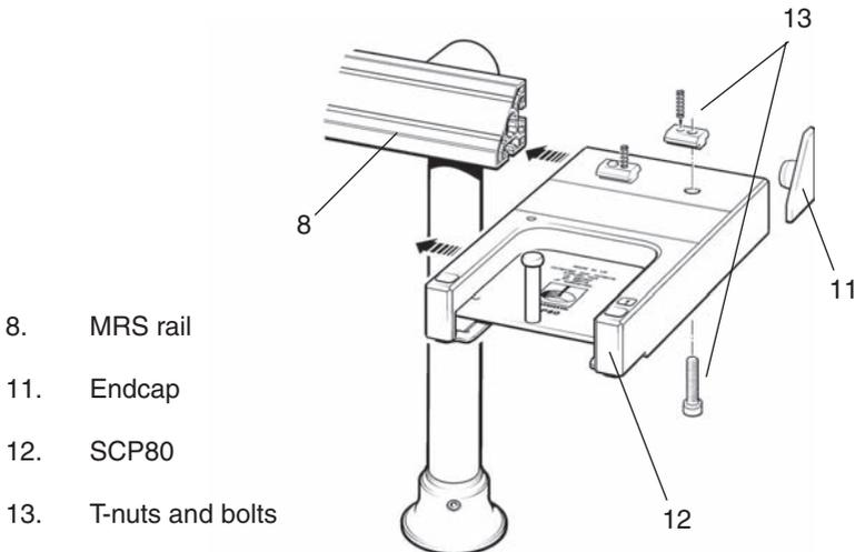
**Figure 19** - Mounting the SCP80 to the MRS rail
