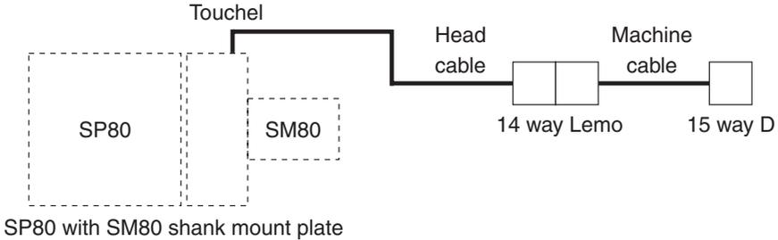
**Figure 24** - Connecting SP80 > SM80 > head cable > machine cable
