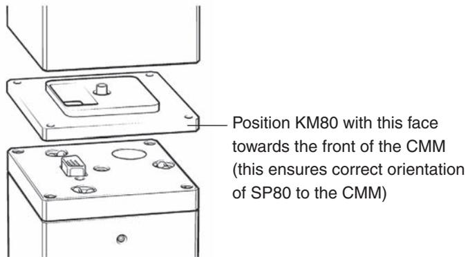
Figure 11 - Orientation and attachment of the KM80 to the quill
