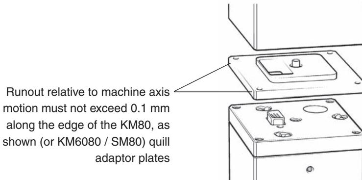
**Figure 21** - Aligning the KM80 with the CMM axes
