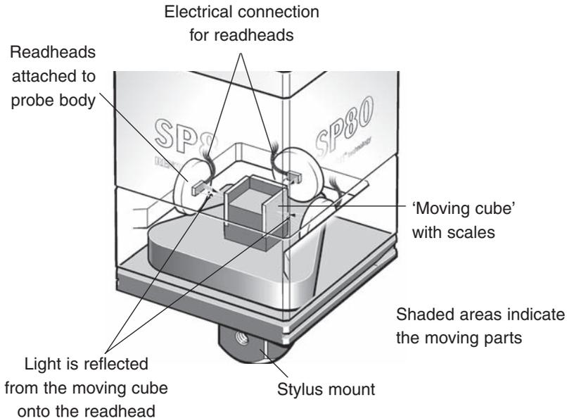
**Figure 9** - Isolated optical metrology principle
