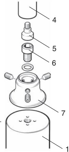
Figure 17 - Connecting the standard leg to the heavy duty leg
