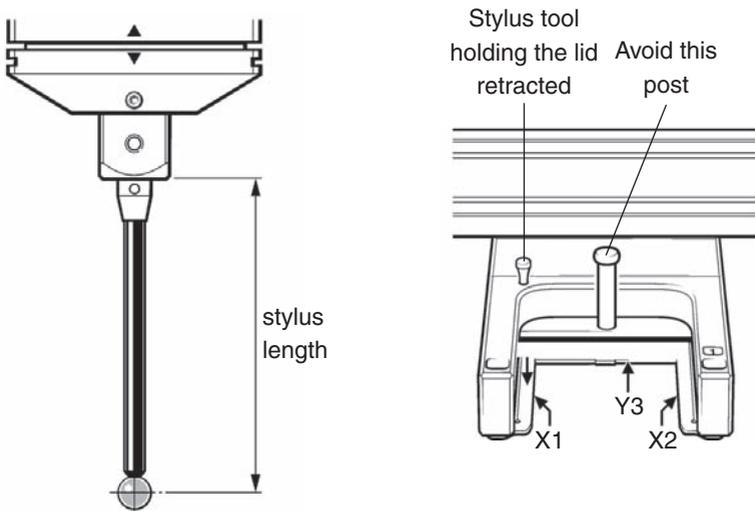
**Figure 29** – Illustrations relating to port datuming procedure
