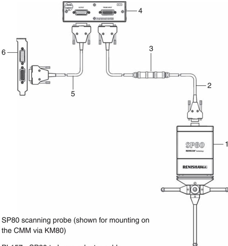
1. SP80 scanning probe (shown for mounting on the CMM via KM80)
