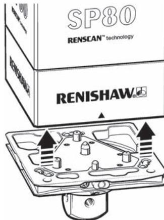
Figure 13 - Mounting the SH80 on the SP80 body
