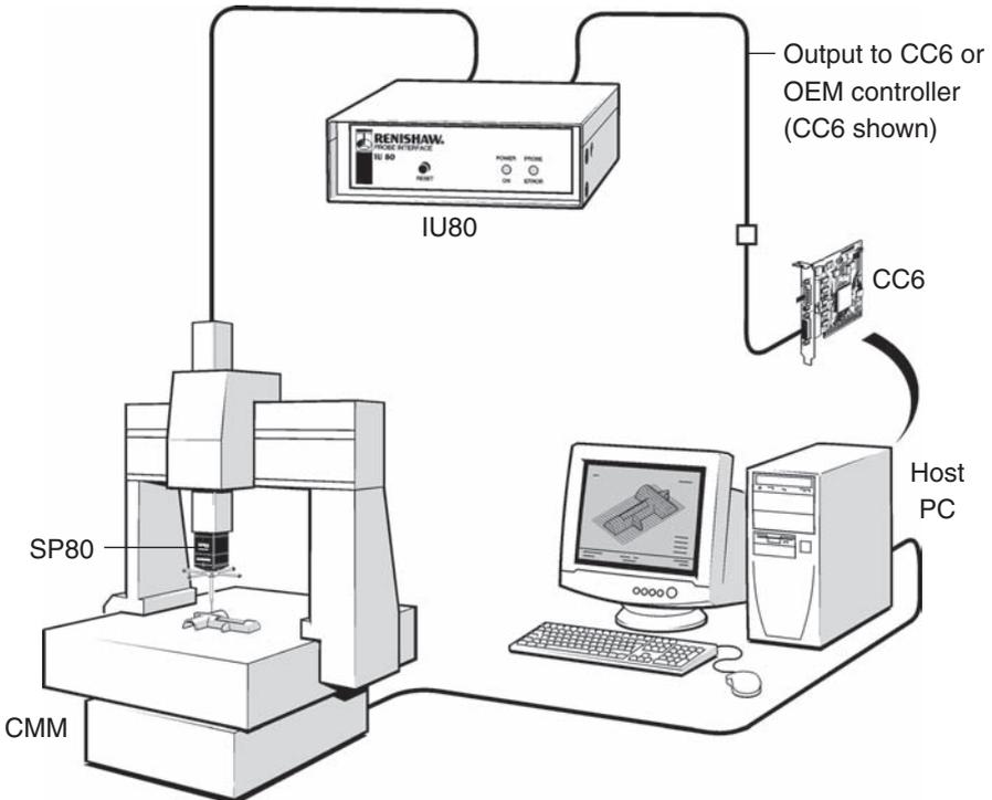
Figure 22 - SP80 integration (with IU80 and CC6)
