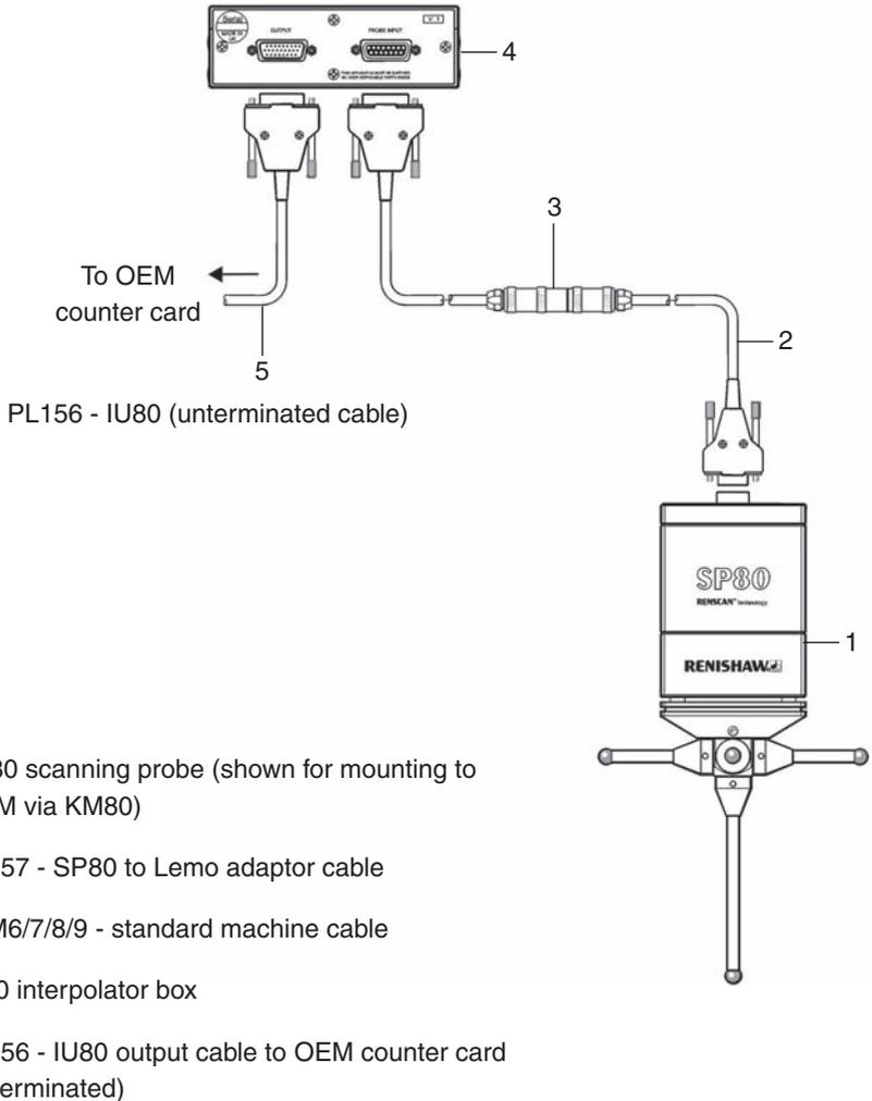
**Figure 28** - Interconnecting SP80 to IU80 and OEM counter card
