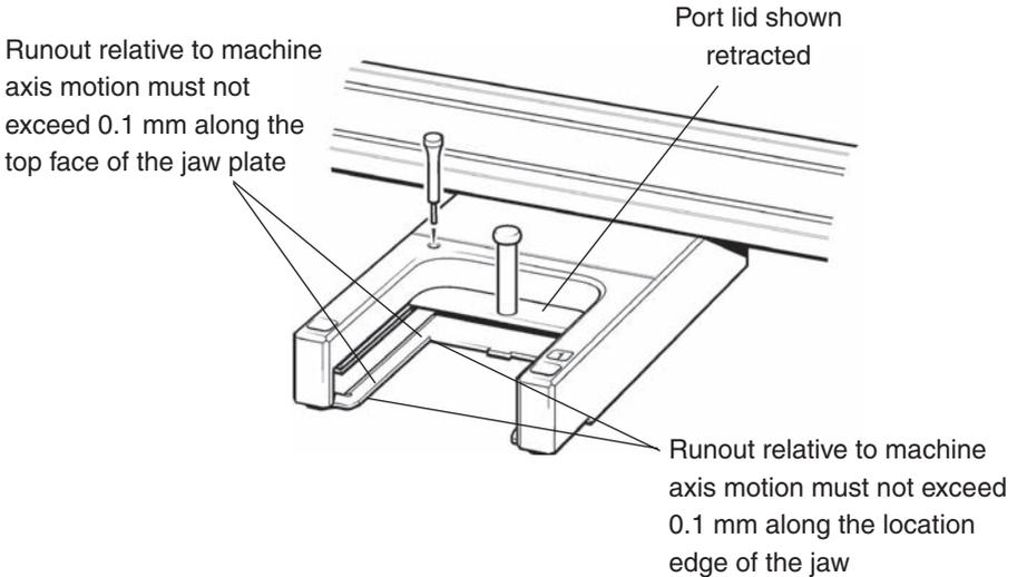
**Figure 20** - Alignment of SCP80 to the CMM axes
