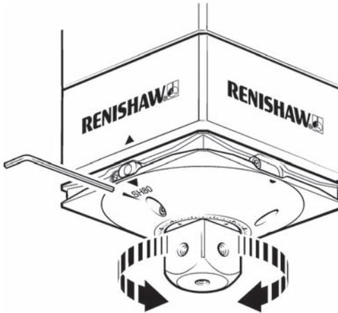
Figure 14 - Rotational stylus adjustment
