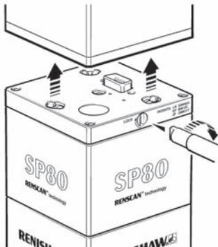
Figure 12 - Attaching the SP80 to the quill adaptor plate (KM80 shown)
